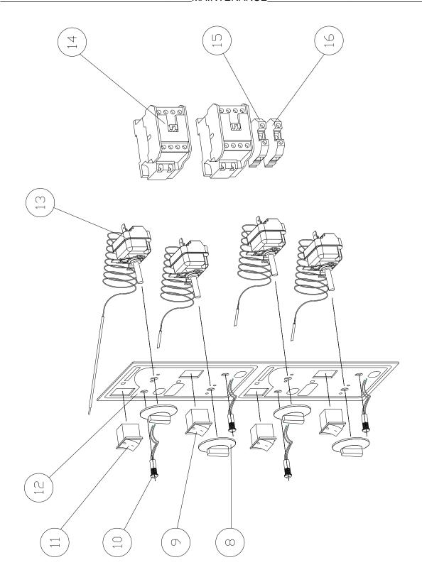
Figure 10-5 Exploded view of electrical parts
